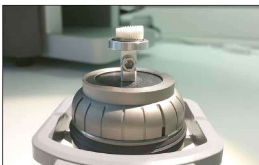
Fig 1 Implant sample mounted on SEM sample holder in cleanroom environment.
