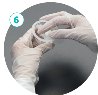
Carefully apply light pressure to stabilise the white insert.
